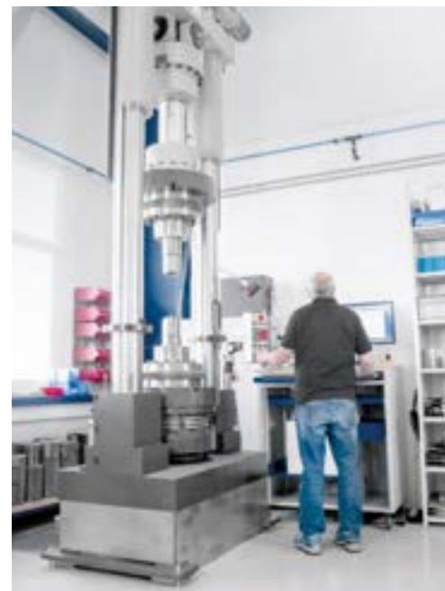
Configuration for rotating torque sensors measurement
